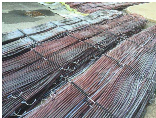
Discolouration of the PFA tubes due to fly ash contamination.
